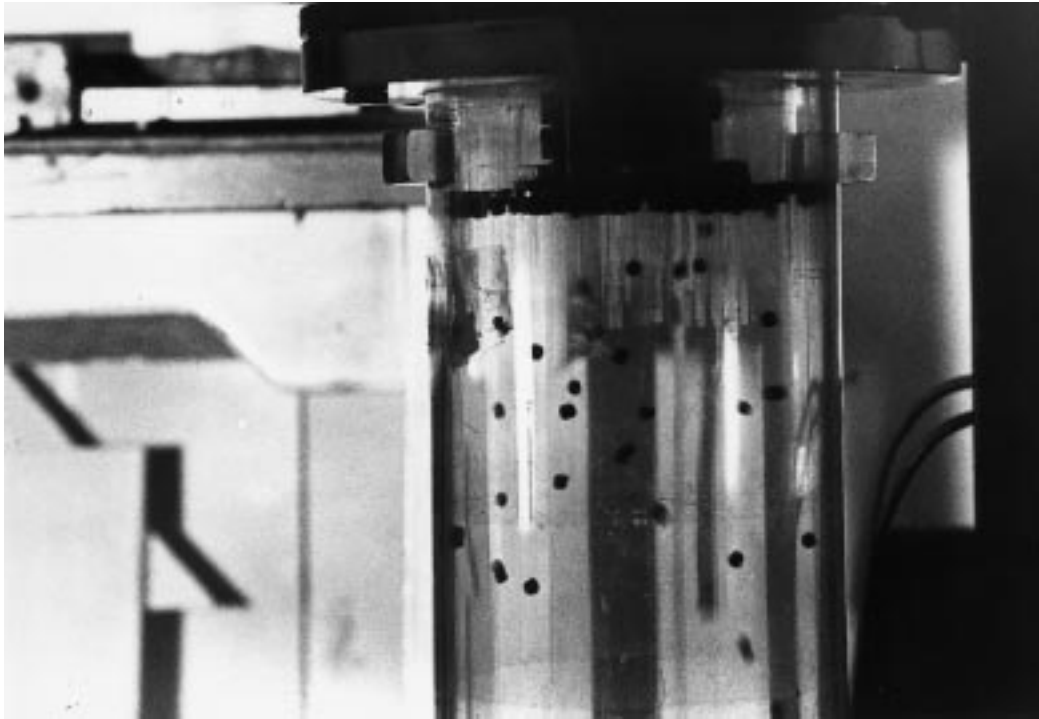
Fig. 5. Photograph of the disperse fluidized regime in a confined volume of the height H = 27 cm, containing one monolayer of glass beads (restitution coefficient e = 0.89 ) of diameter 3.4 mm; air velocity 15 m/s.
